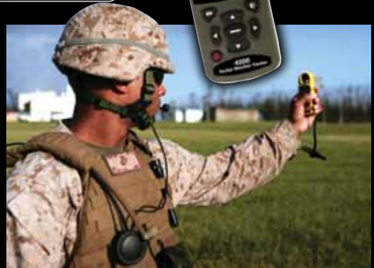
A Marine sergeant utilizes a Kestrel device to measure wind direction, elevation, barometric pressure and wind estimates, and then relays those measurements to the pilots of the KC-130J Super Hercules cargo airplanes.
